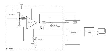
Figure 3-3. Lab Setup to Simulate Temperature Measurement
