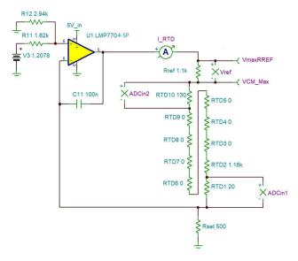
Figure 3-1. TIDA-060042 Schematic
