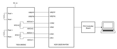
Figure 2-2. Connection Between TIDA-060042 and ADS1282EVM-PDK
