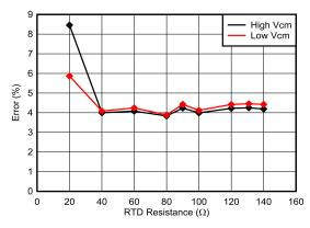
Figure 3-5. Temperature Measurement Accuracy with I<sub>RTD</sub> = 0.5 mA
