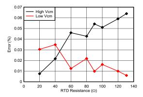
Figure 3-7. Temperature Measurement Accuracy with I<sub>RTD</sub> = 1.5 mA
