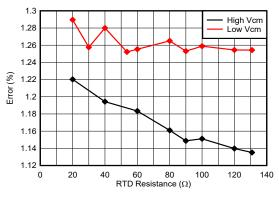
Figure 3-6. Temperature Measurement Accuracy with I<sub>RTD</sub> = 1 mA
