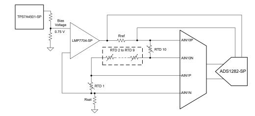
Figure 2-1. Temperature Sensing Application Block Diagram
