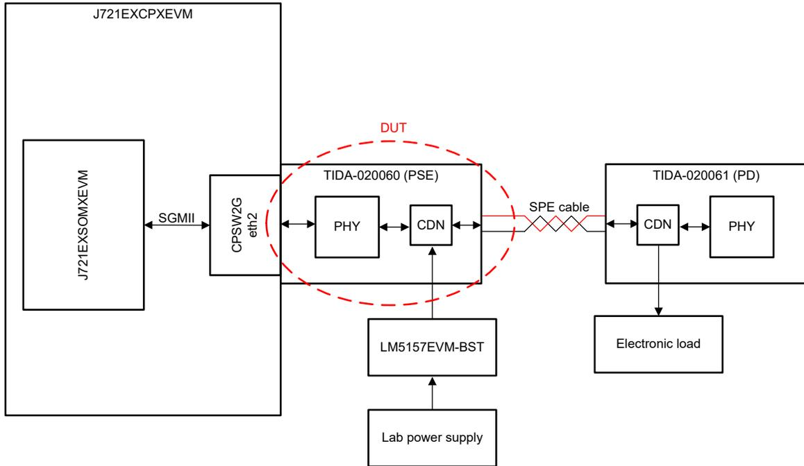
Figure 4-1. Test Setup of SQI Test
