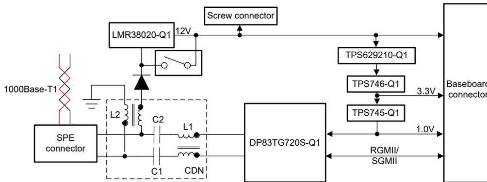
Figure 2-2. TIDA-020061 (PD) Block Diagram
