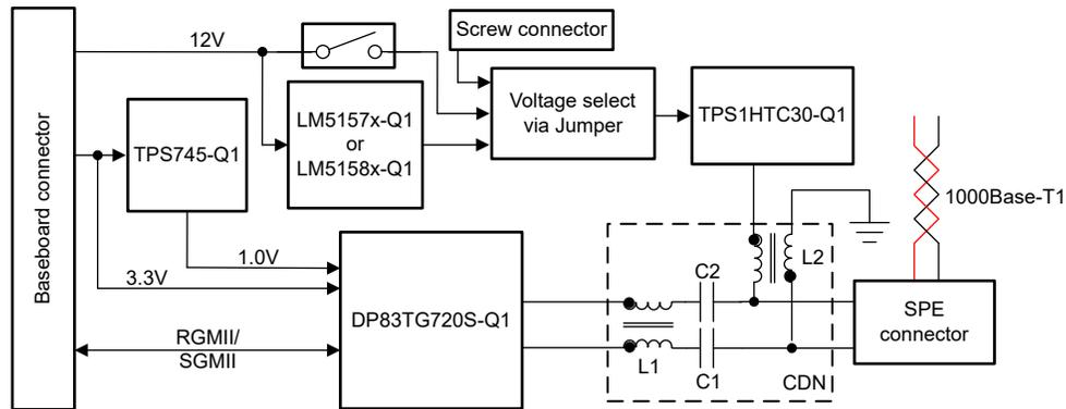
Figure 2-1. TIDA-020060 (PSE) Block Diagram
