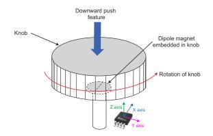
**Use cases:** High-resolution knobs and dials, robotic systems wheels **Recommended devices:** TMAG5170, TMAG5170D, TMAG5273,
