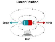
Output signal, either analog or digital, proportional to the magnetic flux density to detect absolute position or angular movements.
