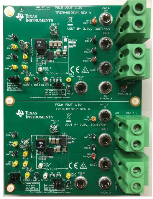
Figure 4-2. TPS7H4010-SEP Board Top View
