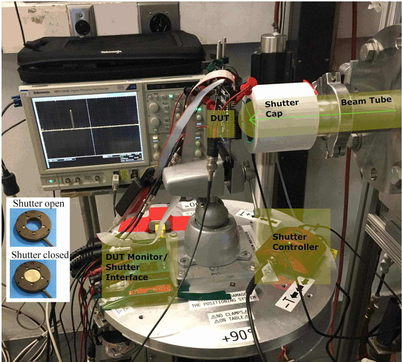
Figure 5. Photograph of the MSP430FR5969-SP Mounted in Front of the Heavy-Ion Beam Exit Port at the Texas A&M Cyclotron
