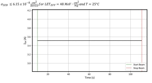
Figure 7-2. Current vs Time for Run # 4 (Enabled) for the TPS7H2211-SEP at T = 25°C
