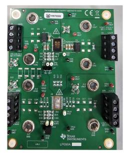
Figure 3-2. TPS7H2211-SEP Board Top View
