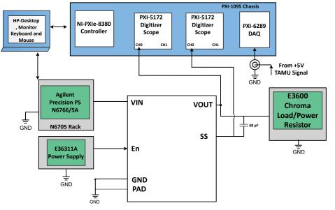
Figure 6-1. Block Diagram of SEE Test Setup With the TPS7H2211-SP
