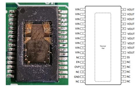
Figure 3-1. Photograph of Delidded TPS7H2211-SEP (Left) and Pin Out Diagram (Right)
