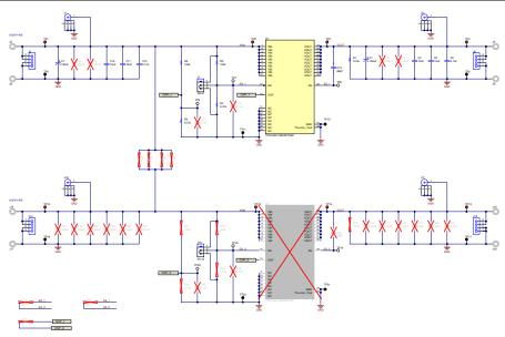
Figure 3-3. TPS7H2211-SEP EVM Schematic
