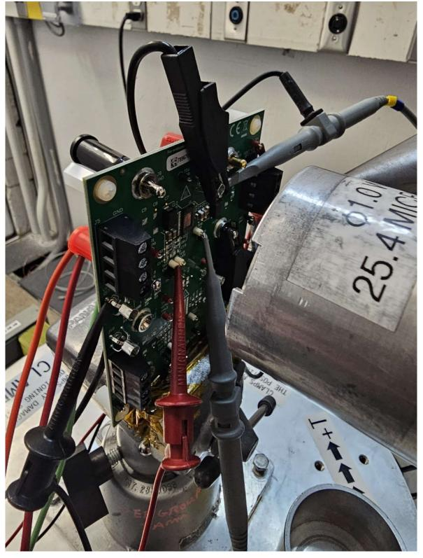
Figure 4-1. Photograph of the TPS7H2211-SEP Evaluation Board Mounted in Front of the Heavy-lon Beam Exit Port at the Texas A&M Cyclotron
