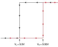
3. With the non-inverting input pin of the comparator labeled as V<sub>TH</sub> and the comparator output in a logic low state (ground), derive an equation for V<sub>TH</sub> where V<sub>H</sub> represents the load voltage (V<sub>LOAD</sub>) when the comparator output transitions from low to high. Note that the simplified diagram for deriving the equation shows the comparator output as ground (logic low).
