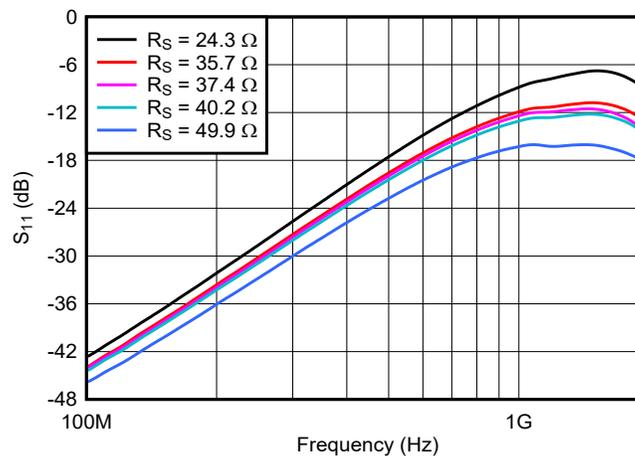
**Figure 11.  $S_{11}$  with Varying  $R_S$**
