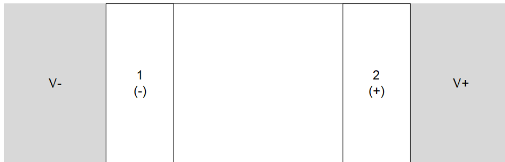
Figure 8-14. Recommended Layout: DEC Package
