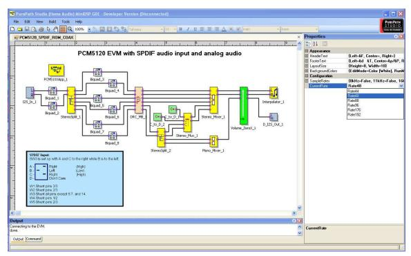
Figure 18. PurePath Studio Sample Rate Control
