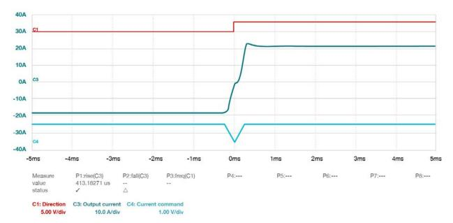
Figure 3. Current waveform during the transition from discharge to charge mode.
