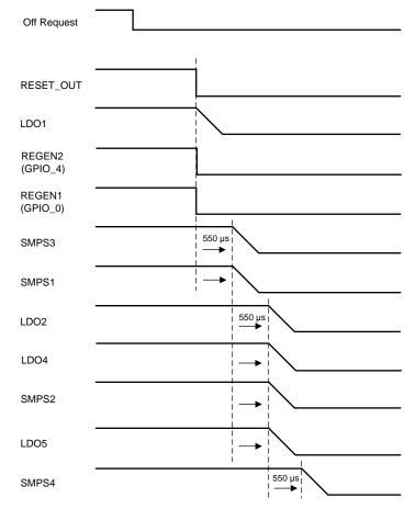
Figure 8. Power Down Sequence of TPS659163RGZR
