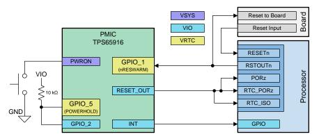
Figure 3. Reset Connections With PWRON Configuration
