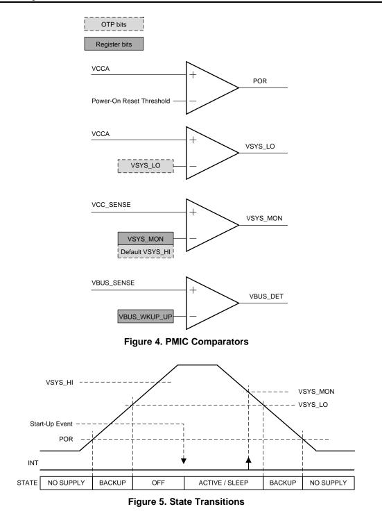
**NOTE:** The maximum input voltage of the VCC\_SENSE pin depend on the OTP setting of PMU\_CONFIG [HIGH\_VCC\_SENSE] as listed in the *Recommended Operating Conditions* table of the TPS65916 data sheet. This configuration is set as HIGH\_VCC\_SENSE = 0 with the VCC\_SENSE and pins are connected to VCCA.
