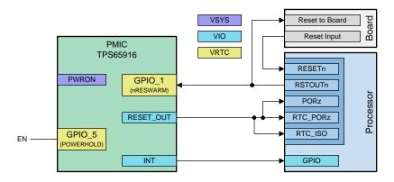
Figure 2. Reset Connections With POWERHOLD Configuration
