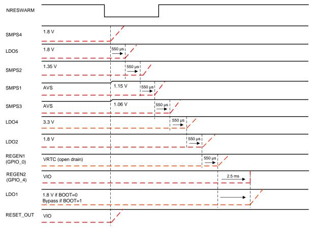
Figure 9. Warm Reset Sequence of TPS659163RGZR
