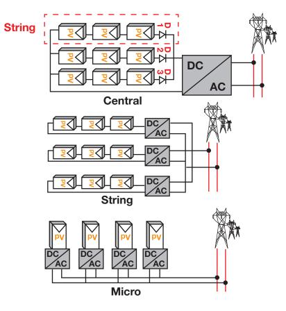
Figure 1. Different inverter configurations.
