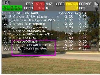
Example application of VLIB providing ~10X pixel processing improvement over standard C code
