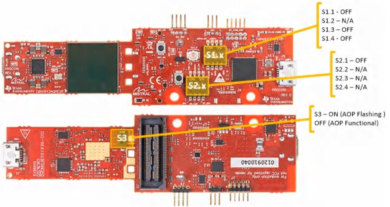
**Figure 5-12. Switch Configuration for Modular Mode**
