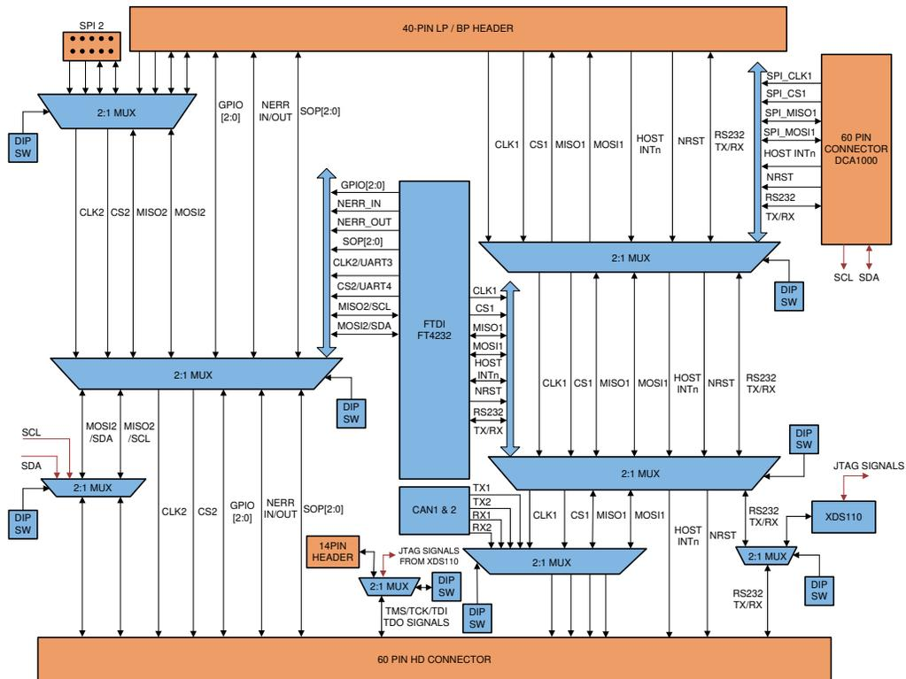
Figure 2-4. Muxing Scheme
