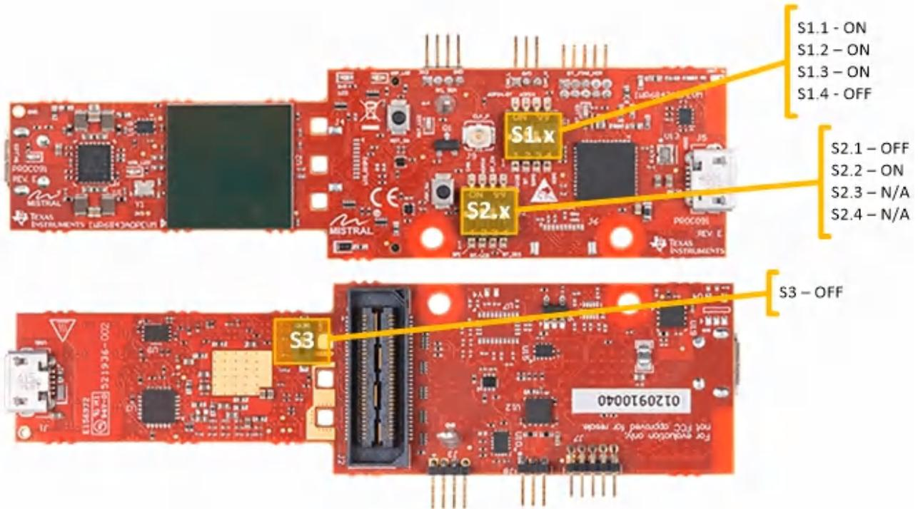
**Figure 5-15. Switch Configuration for MMWAVEICBOOST Mode**
