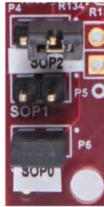
Figure 2-24. SOP Jumpers
