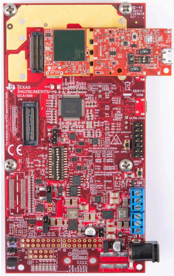
For mounted mode, the UART should be routed to the 60-pin connector. Set up the device as shown in [Figure 7-10](#). When mounted as shown, the SOP mode is overridden by the MMWAVEICBOOST SOP configuration.
