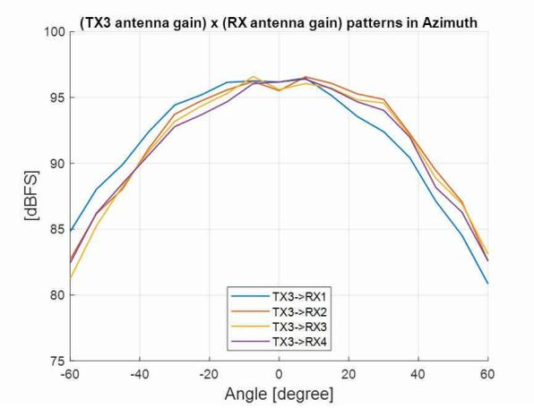
**Figure 3-12. TX3 Antenna Radiation Pattern in Azimuth**
