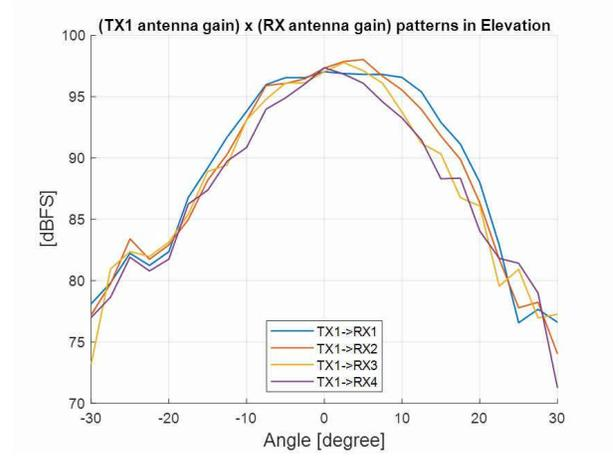
**Figure 3-13. TX1 Antenna Radiation Pattern in Elevation**
