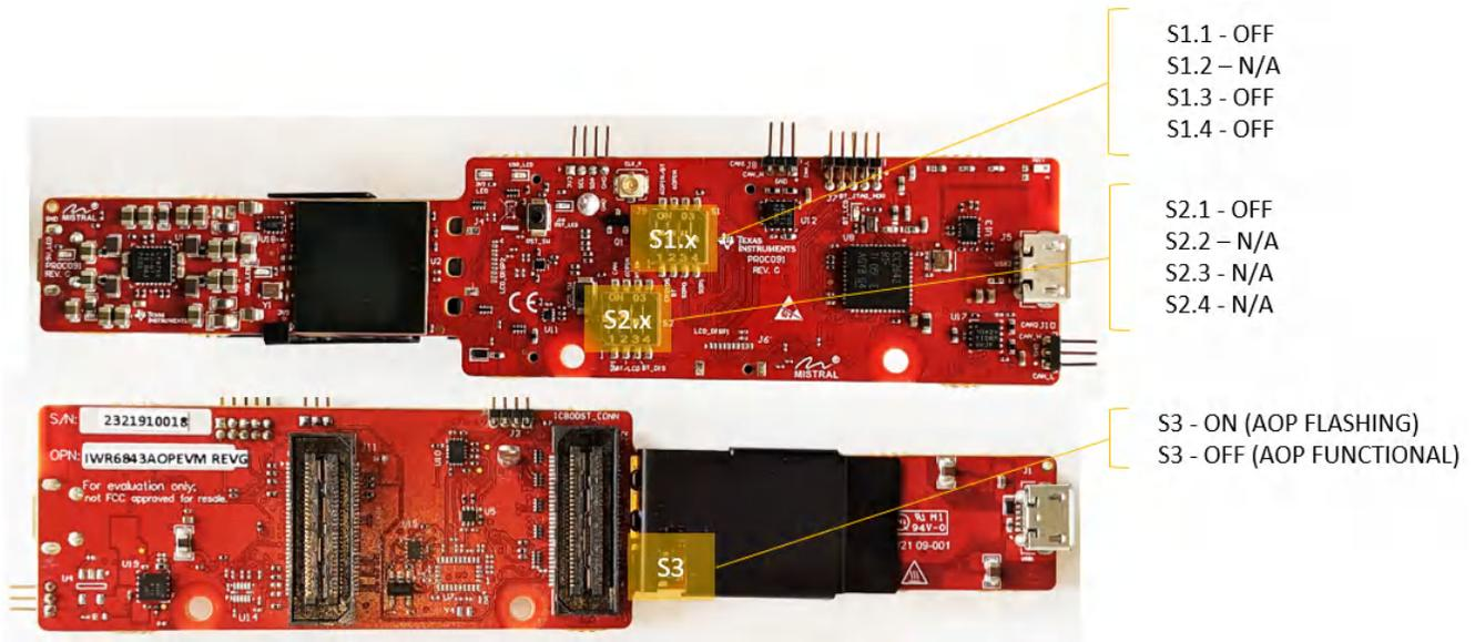
**Figure 4-12. Switch Configuration for Modular (USB) Mode**
