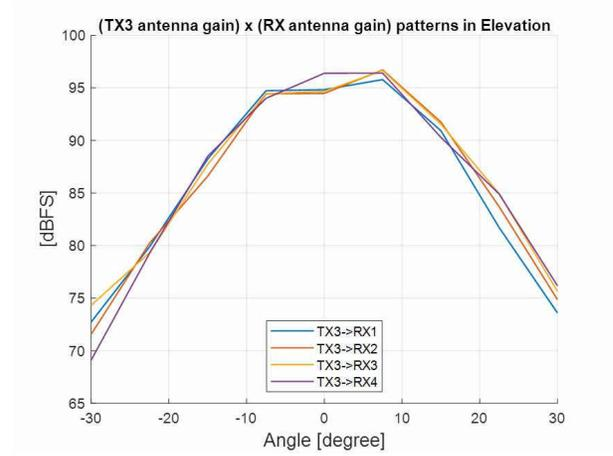
**Figure 6-13. TX3 Antenna Radiation Pattern in Elevation**
