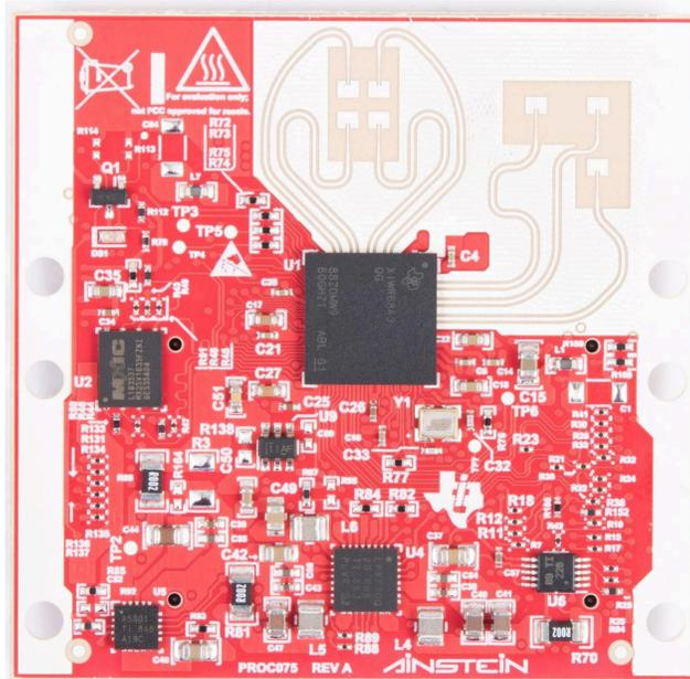
Figure 6-3. PCB Antenna – Top
