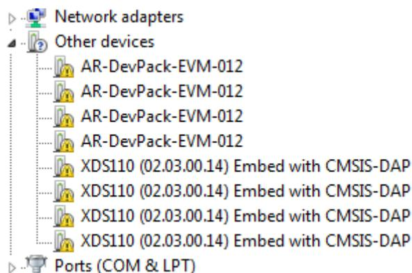
**Figure 2-8. Uninstalled Devices**
