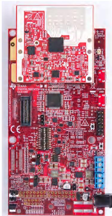
**Figure 2-10. Integration of MMWAVEICBOOST and Starter Kit**
