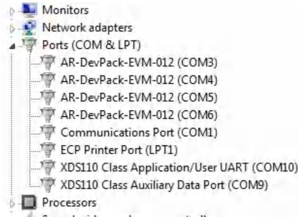
**Figure 2-9. COM Ports After the Driver Installation**
