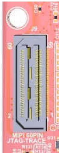
**Figure 2-20. 60-Pin MIPI Connector**
