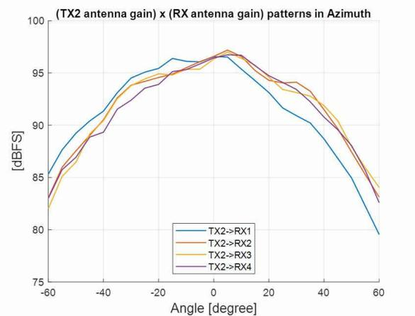
**Figure 6-9. TX2 Antenna Radiation Pattern in Azimuth**
