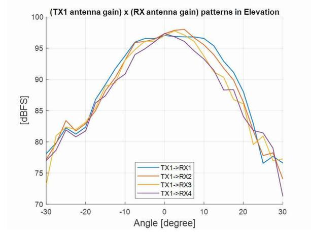
**Figure 6-11. TX1 Antenna Radiation Pattern in Elevation**
