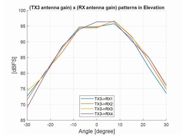
**Figure 3-15. TX3 Antenna Radiation Pattern in Elevation**
