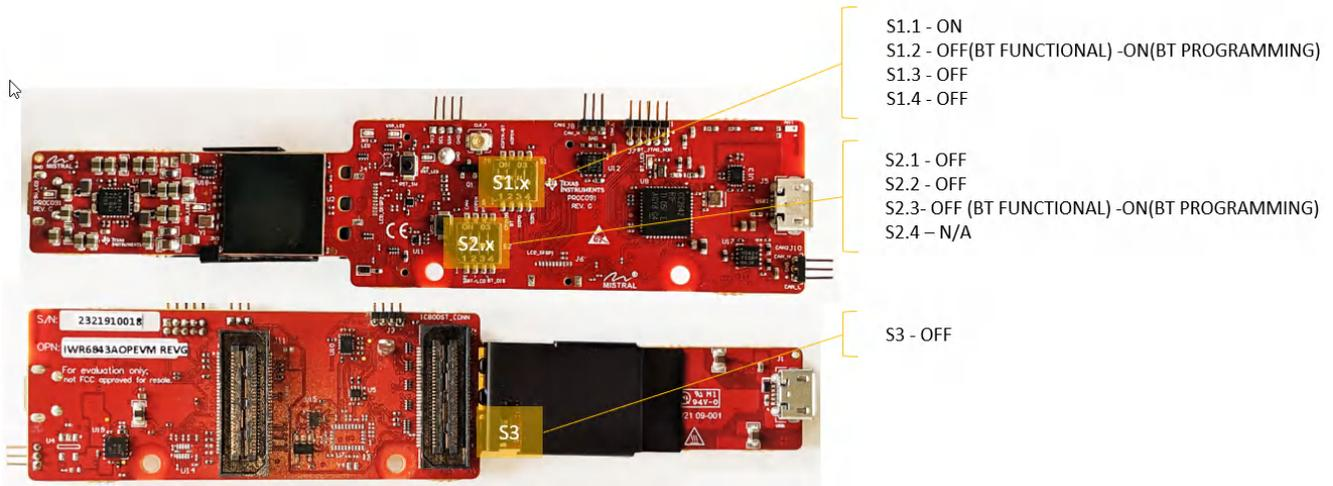
**Figure 4-13. Switch Configuration for Modular (Bluetooth) Mode**
