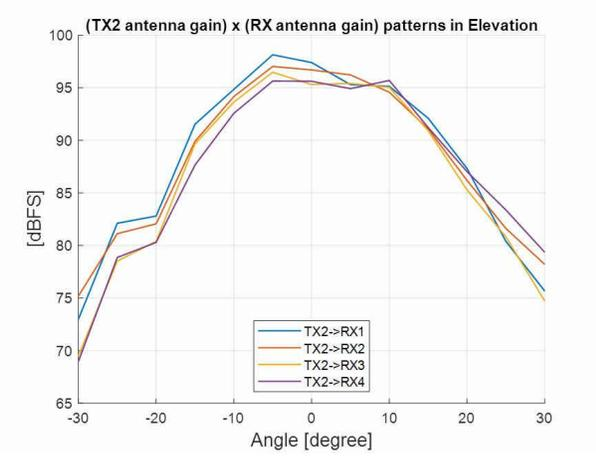
**Figure 3-14. TX2 Antenna Radiation Pattern in Elevation**
