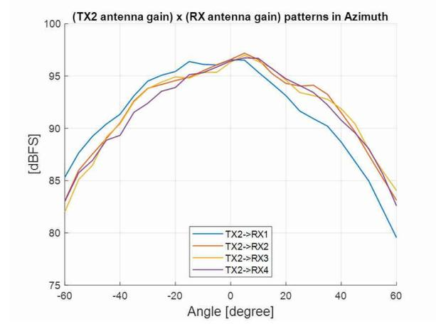
**Figure 3-11. TX2 Antenna Radiation Pattern in Azimuth**
