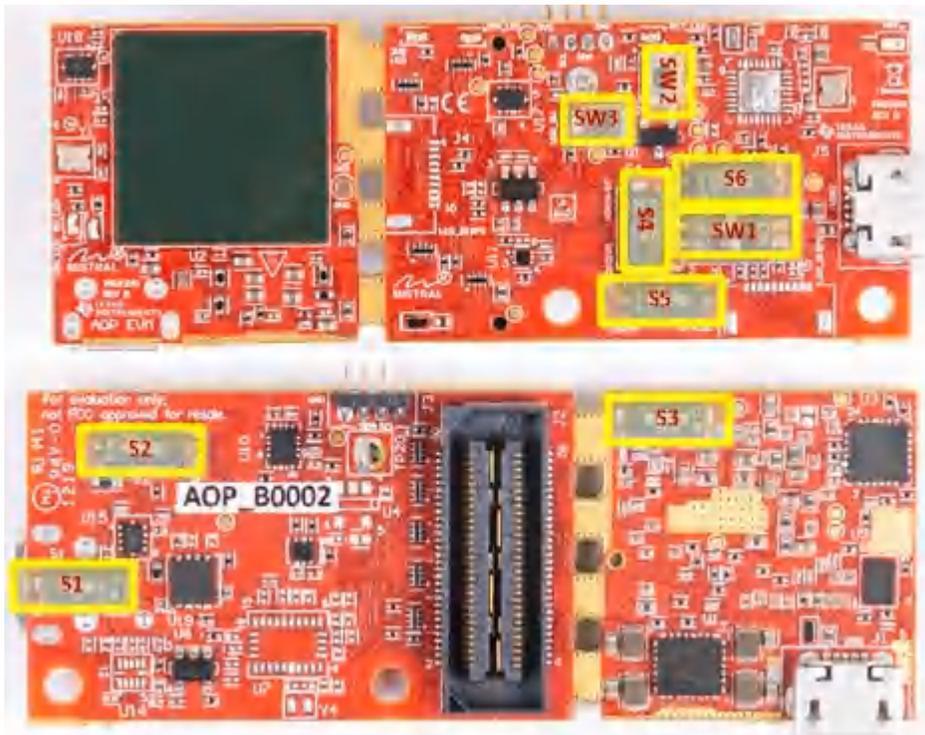
**Figure 7-7. IWR6843AOPEVM Switches**
