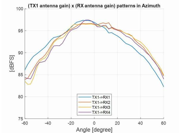
**Figure 6-8. TX1 Antenna Radiation Pattern in Azimuth**
