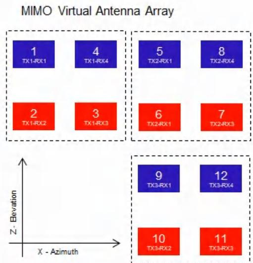
RX2 and RX3 are  $180^\circ$  out of phase with respect to RX1 and RX4. Because of this, a  $180^\circ$  phase inversion needs to be applied in software processing for the corresponding virtual RX channels (highlighted in Red)
