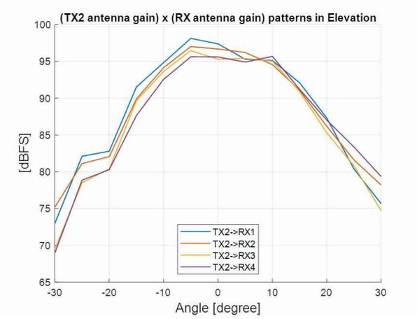
**Figure 6-12. TX2 Antenna Radiation Pattern in Elevation**
