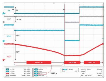
Figure 2. TPS61094 Power-cycle Measurements
