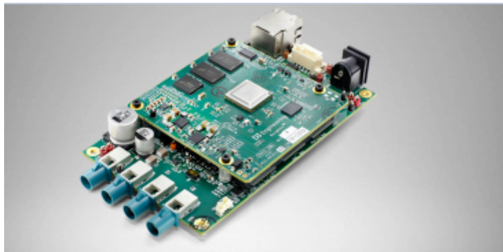
Figure 1. The TDA3x Automotive Starter Kit Helps Simulate Challenging Scenes to Enable Algorithm Development and Turning under Controlled Circumstances
