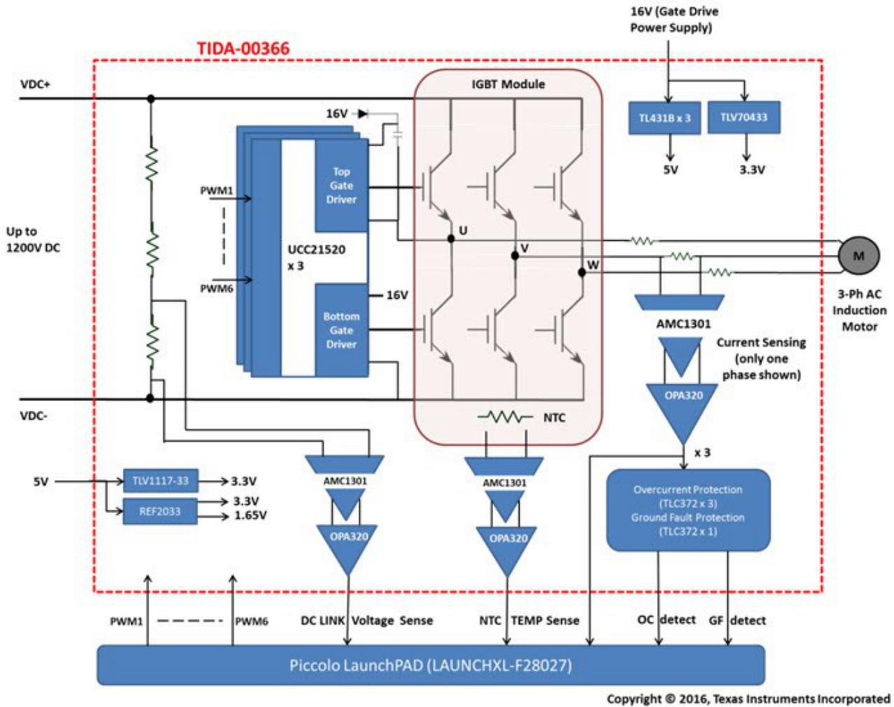
**Figure 1. High-level Block Diagram of TIDA-00366**
