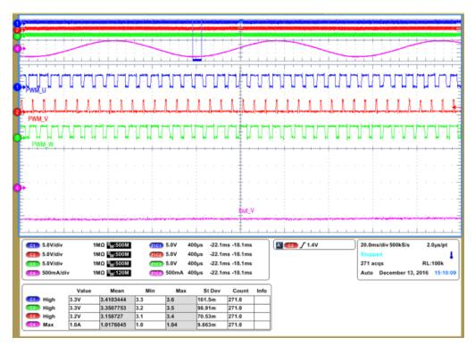
Figure 13. IN2 (PWM\_V) 10% DC, Output Phase V at 270°
