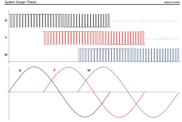
Figure 5. PWM Scheme for Sine Waveform Output
