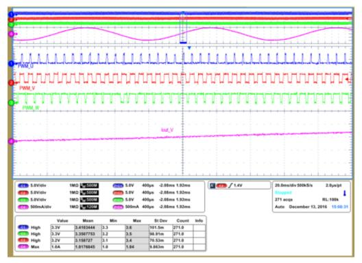
Figure 11. IN2 (PWM\_V) 50% DC, Output Phase V at 0°
