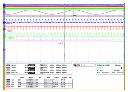
Figure 12. IN2 (PWM\_V) 90% DC, Output Phase V at 90°
