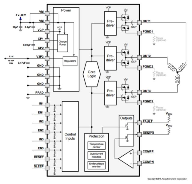
Figure 1. DRV8313 Block Diagram
