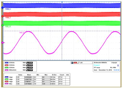
Figure 9. Three PWM Input Signals and Current Output Phase U
