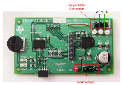
Figure 6. Input and Output Connections
