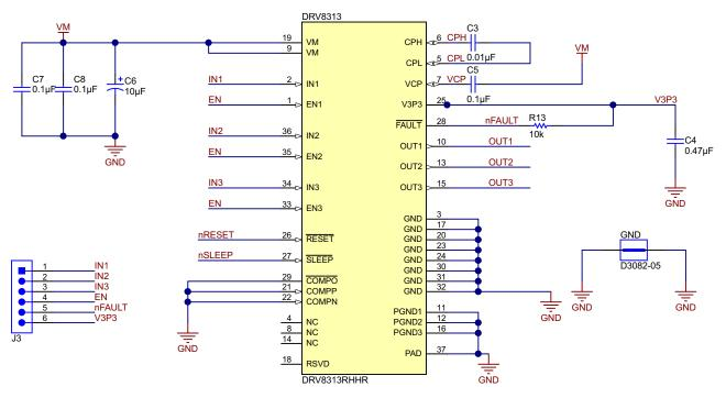
The three phases of the motor are driven by the three outputs of the DRV8313, as Figure 3 shows.
