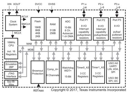
Figure 2. MSP430G2553 Functional Block Diagram
