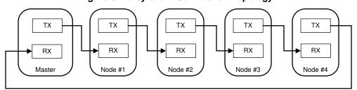
Figure 3. Daisy-chain Connection Topology
