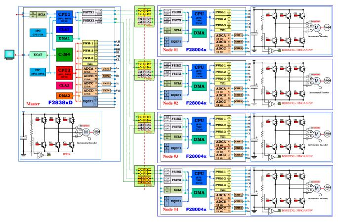
Figure 1. TIDM-02006 System Block Diagram
