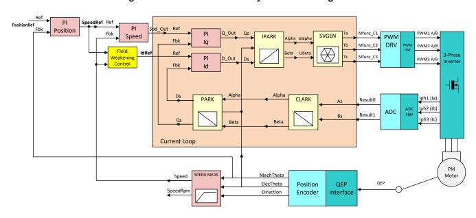
Figure 2. Servo Drive Control System Block Diagram
