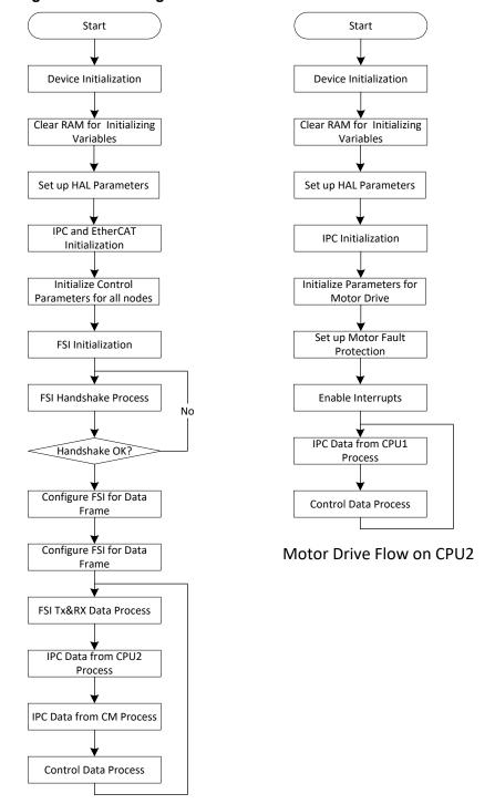
Figure 11. Main Program Flowchart on CPU1 and CPU2 of F2838x
