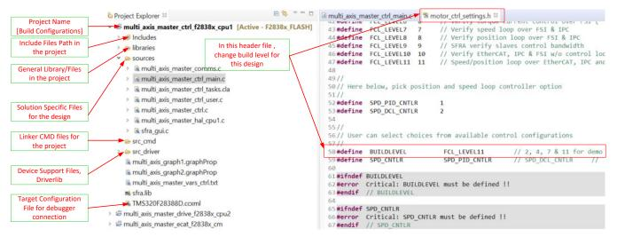
Figure 18. Project Explorer View of Master Control Project
