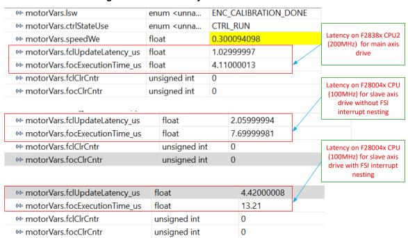
Figure 33. PWM latency and FOC execution time
