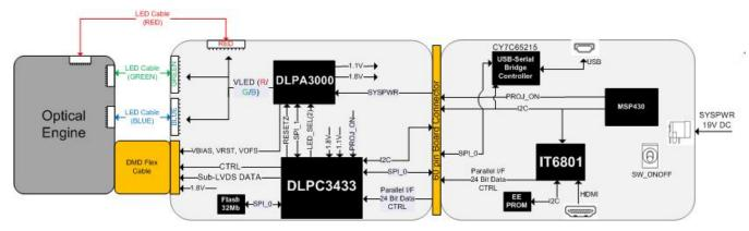
Figure 2. DLP LightCrafter Display EVM Block Diagram
