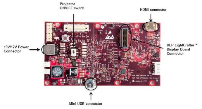
Figure 5. DLP LightCrafter Display Main Board
