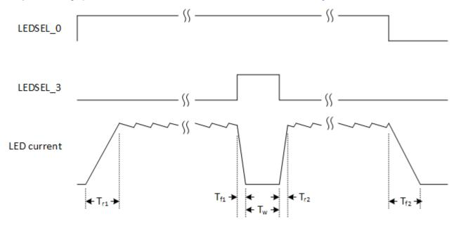
Figure 4. DLP5531-Q1 Electronics EVM LED Driver Board Timing Specifications
