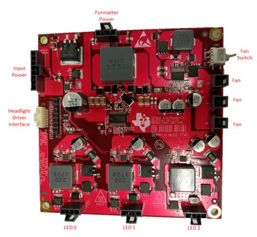
Figure 2. DLP5531-Q1 EVM LED Driver Board
