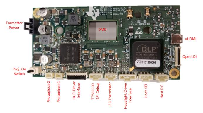
Figure 1. DLP5531-Q1 EVM Formatter Board
