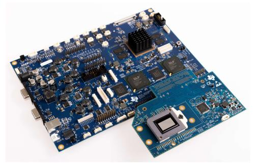
Figure 2-5. EVMs Connected
