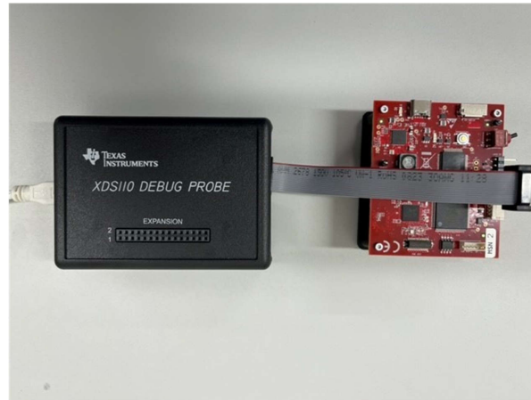
Figure 4-3. XDS110 Debug Probe and Board Assembly
