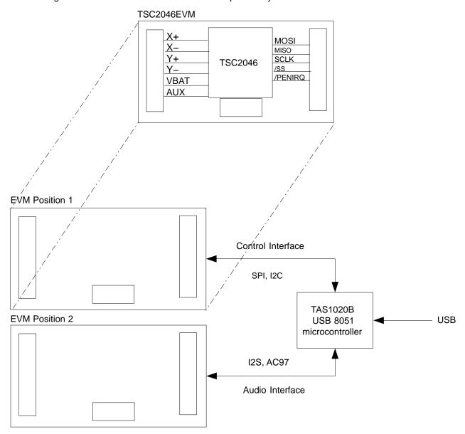
Figure 1. TSC2046EVM-PDK Block Diagram
