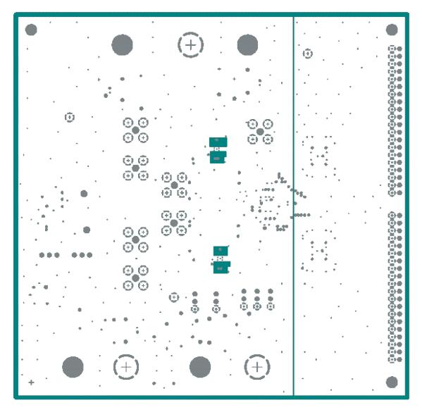
Figure 5. Layer 5, Ground Plane
