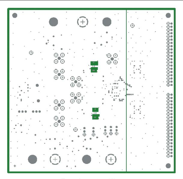
Figure 2. Layer 2, Ground Plane
