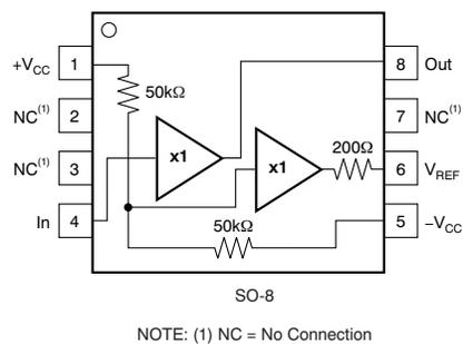
**Figure 1. Buffer Pinout Compatible with DEM-BUF-SO-1A**
