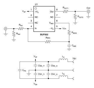
Figure 2. Schematic
