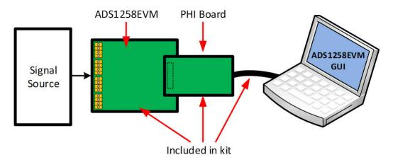
Figure 1-1. System Connection for Evaluation
