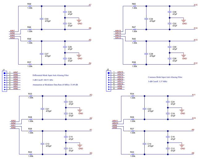
Figure 3-1. ADS1258EVM Analog Input Channels and Filtering
