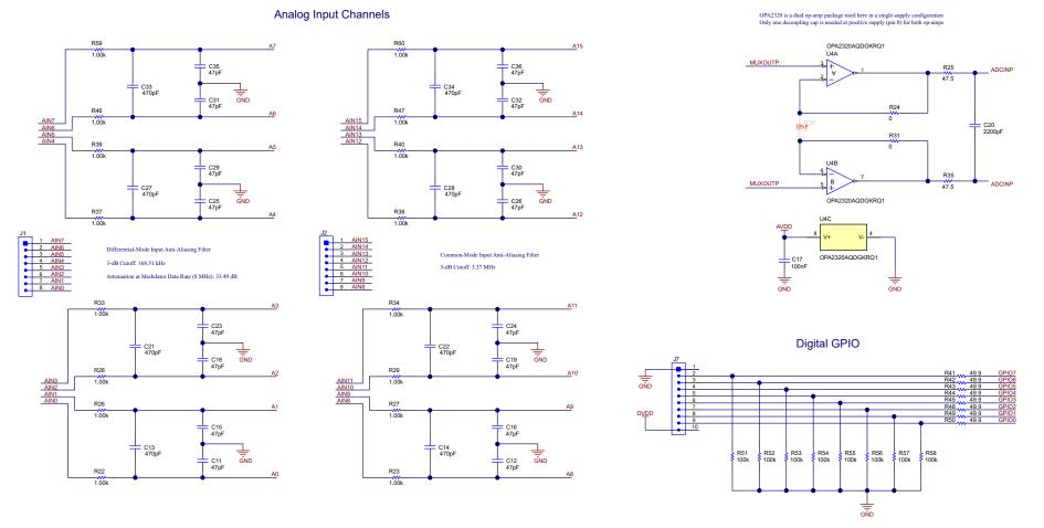
Figure 8-3. ADS1258EVM Analog Input, Multiplexer Loop, and GPIO Circuits
