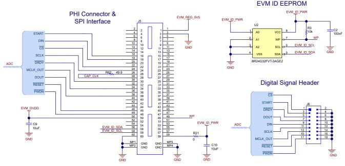
Figure 4-1. ADS1258EVM Digital Interface Connections (SPI and I<sup>2</sup>C)
