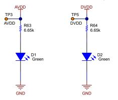
Figure 5-2. ADS1258EVM AVDD and DVDD Indicator LEDs
