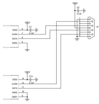
Figure 2. Power and Digital Outputs
