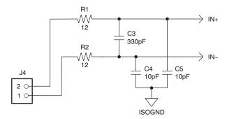
Figure 1. AMC1204EVM Schematic: Analog Input Section
