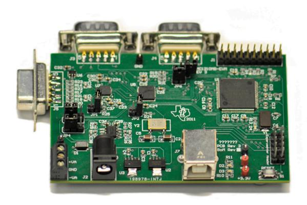
This user's guide describes the characteristics, operation, and use of the  $\underline{\mathsf{AMC1210MB\text{-}EVM}}$  as part of an evaluation system when used with Texas Instruments delta-sigma ( $\Delta\Sigma$ ) modulator evaluation modules (EVMs) in resolver or current-shunt applications. A schematic diagram and bill of materials are included in this document.
