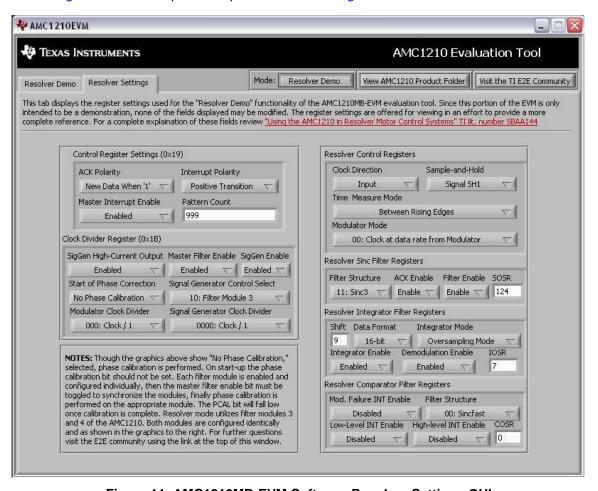
Figure 11. AMC1210MB-EVM Software Resolver Settings GUI
