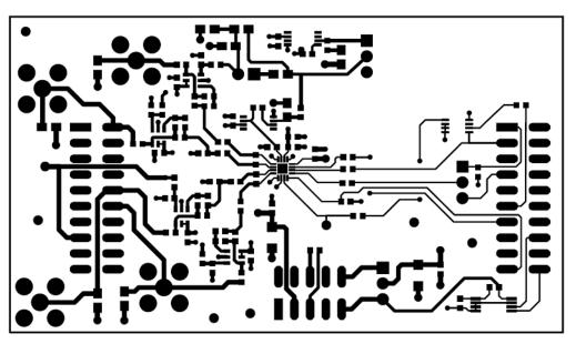
Figure 14. ADS794xEVM PCB: Top Layer
