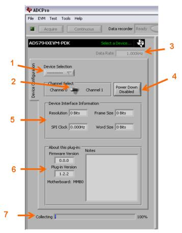
Figure 12. ADS794xEVM Plug-in: Device Configuration Tab
