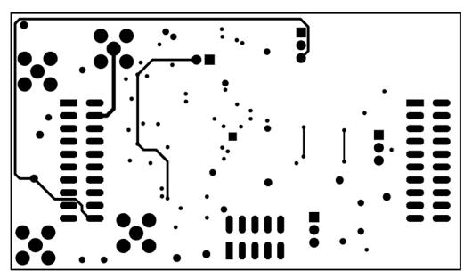
Figure 17. ADS794xEVM PCB: Bottom Layer
