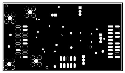
Figure 15. ADS794xEVM PCB: Ground Layer
