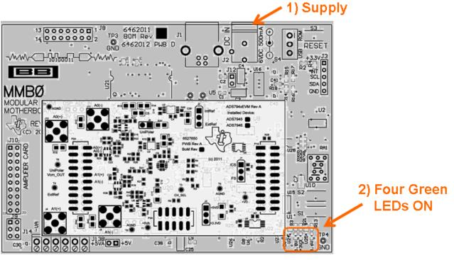
Figure 8. Powering Up ADS794xEVM-PDK
