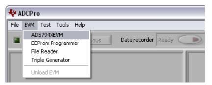
Figure 10. Loading ADS794xEVM Plug-in From ADCPro
