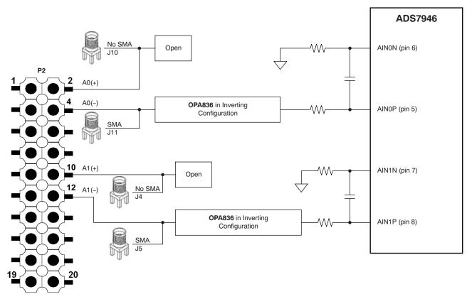
Figure 2. ADS794xEVM and ADS7946 Analog Inputs
