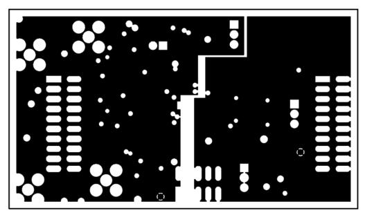
Figure 16. ADS794xEVM PCB: Power Layer
