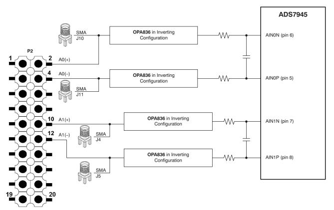
Figure 1. ADS794xEVM and ADS7945 Analog Inputs
