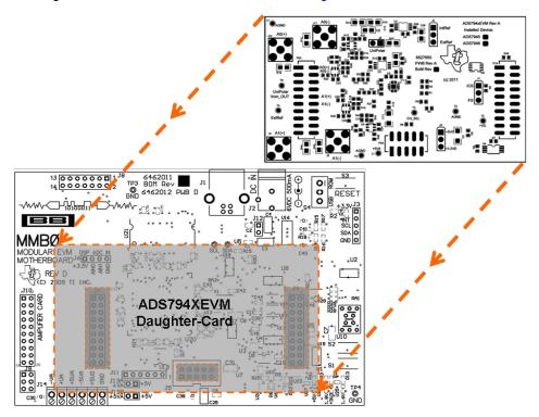
Step 3. Plug the ADS794xEVM into the MMB0, as Figure 7 illustrates.
