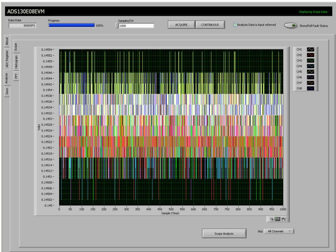
**Figure 18. Eight-Channel Read of Internal Temperature Data**
