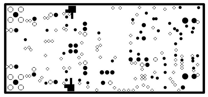
Figure 33. ADSxx53EVM PCB: Ground Layer
