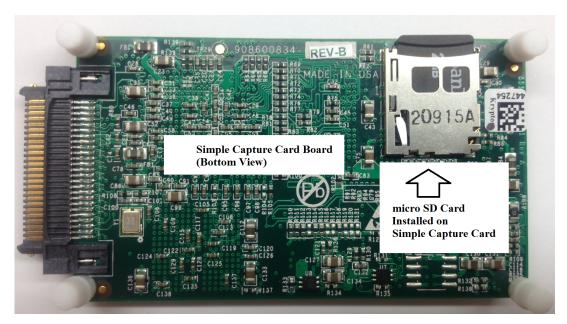
Figure 7. Bottom View of Simple Capture Card Board with microSD Card Installed
