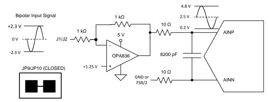
Figure 3. Bipolar Input Signal Configuration with  $2 \times V_{ref}$  range
