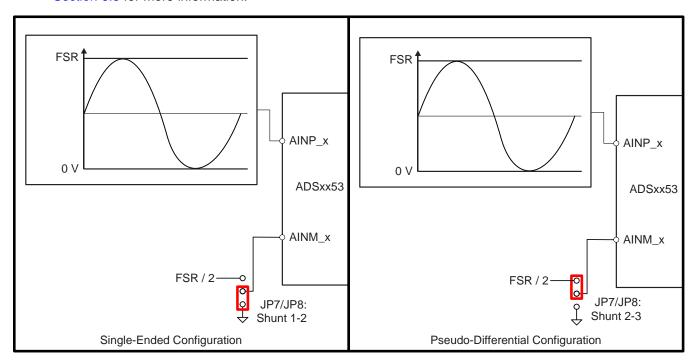
Figure 2. Single-Ended or Pseudo-Differential Input Configuration
