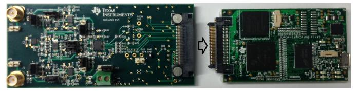
Figure 9. Connecting the ADSxx53EVM Board to the Simple Capture Card Controller Board
