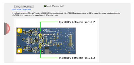
Figure 22. Single-Ended or Pseudo-Differential Jumper Settings Description on the GUI
