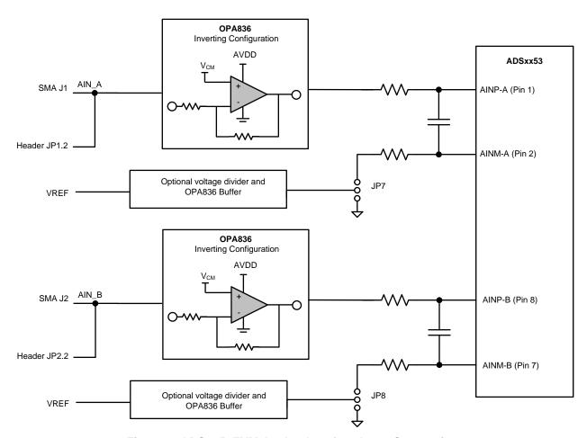
Figure 1. ADSxx53EVM Analog Interface Input Connections
