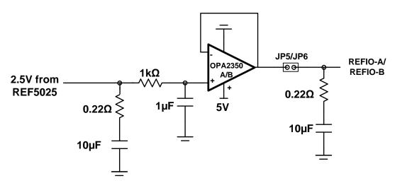
Figure 5. REF5025 2.5-V External Reference Source and OPA2350 Reference Driver
