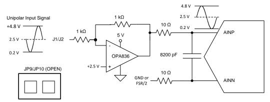
Figure 4. Unipolar Input Signal Configuration
