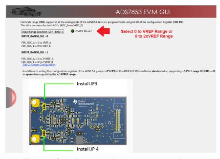
Figure 21. Selecting 0 to  $V_{ref}$  Range or 0 to 2 ×  $V_{ref}$  Range
