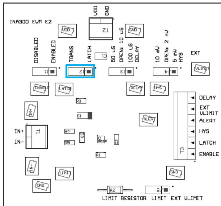
Figure 6. Transparent/Latch Jumper
