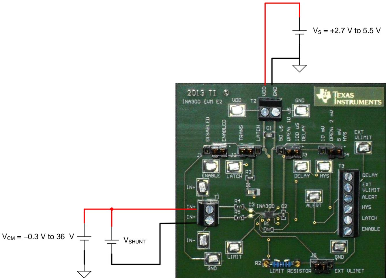
**Figure 2. Connecting the INA300EVM with Voltage Sources**
