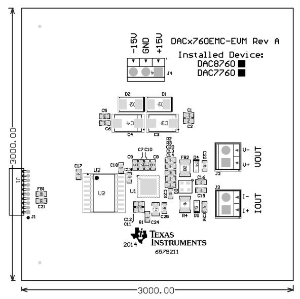
Figure 22. DACx760EMC-EVM Assembly Drawing
