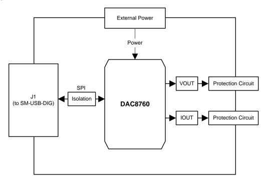
Figure 2. DAC8760EVM Block Diagram
