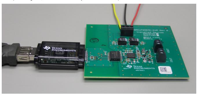
Figure 4. SM-USB-DIG Connection to the DAC8760EVM
