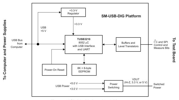
Figure 3. USB-DIG Platform Block Diagram
