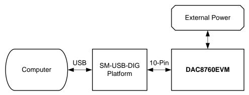
Figure 1. DAC8760EVM Hardware Setup
