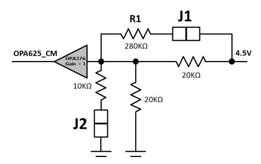
Figure 2. Common Mode Selection Jumpers
