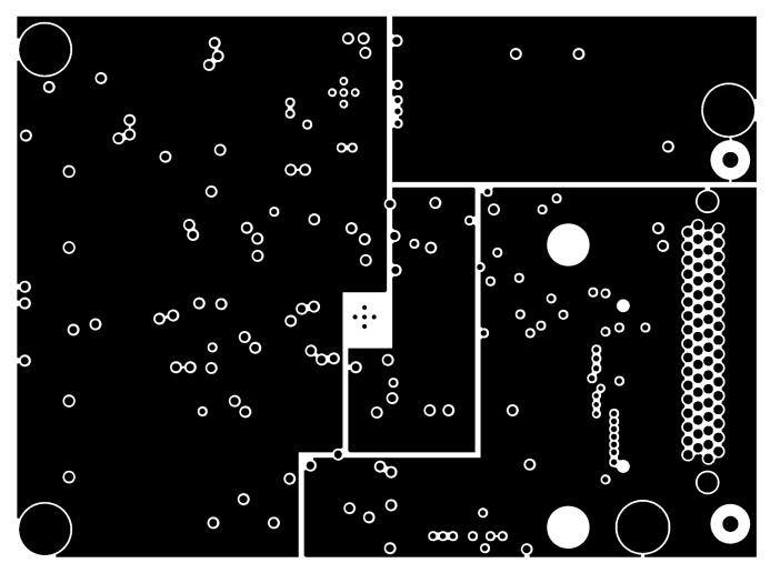
Figure 18. ADS9110EVM PCB Layer 3: Power Planes
