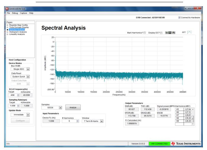
Figure 13. Spectral Analysis Tool
