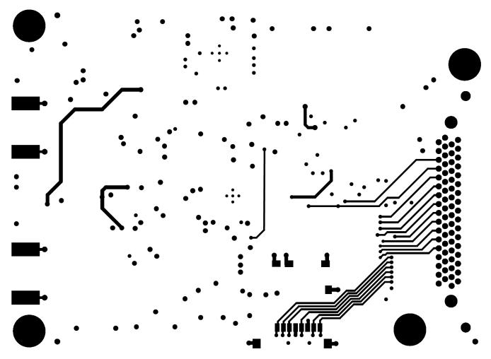
Figure 19. ADS9110EVM PCB Layer 4: Bottom Layer
