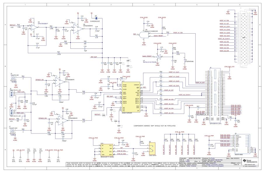
Figure 20. Schematic Diagram (Page 1) of the ADS9110EVM PCB
