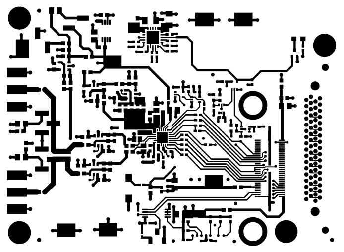
Figure 16. ADS9110EVM PCB Layer 1: Top Layer
