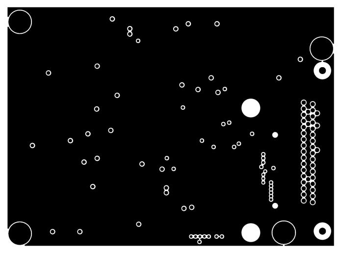
Figure 17. ADS9110EVM PCB Layer 2: GND Plane
