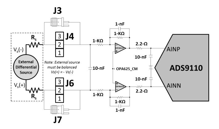
Figure 1. OPA625 Differential Input Driving Path
