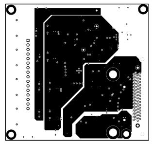
Figure 7-4. ADS8332EVMV2 PCB Layer 3: Power Planes
