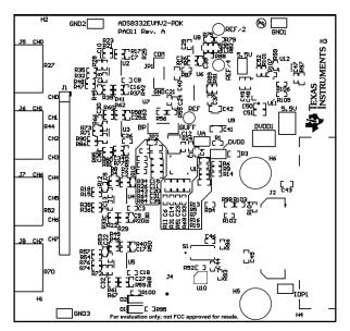
Figure 7-1. ADS8332EVMV2 PCB: Top Overlay
