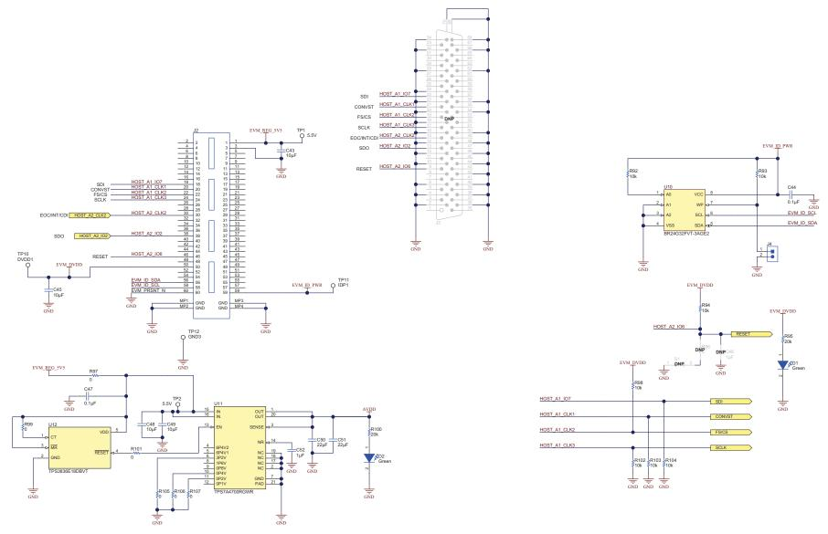
Figure 7-8. ADS8332EVMV2-PDK Schematic: Interface
