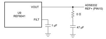
Figure 2-2. REF6041 4.096-V Onboard Reference Source
