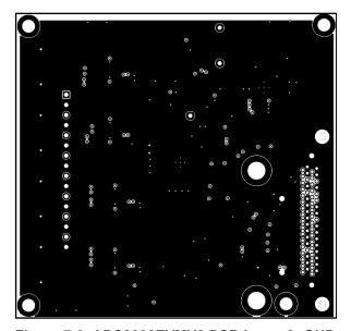
Figure 7-3. ADS8332EVMV2 PCB Layer 2: GND Plane
