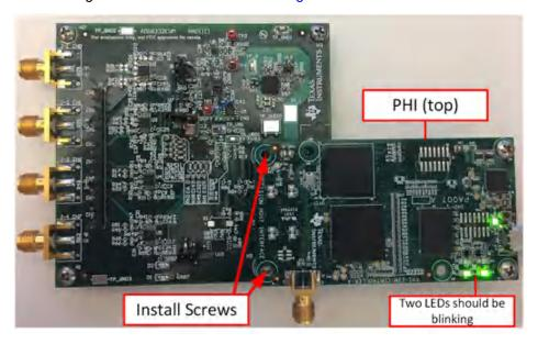
Figure 6-1. ADS8332EVMV2-PDK Hardware Setup and LED Indicators
