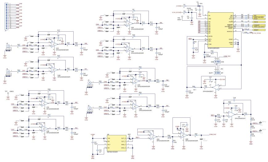
Figure 7-7. ADS8332EVMV2-PDK Schematic: ADC
