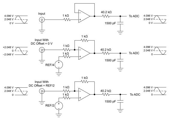
Figure 6-9. Input Amplifier Configuration Examples
