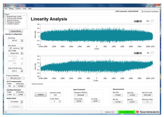
Figure 15. Linearity Analysis Tool
