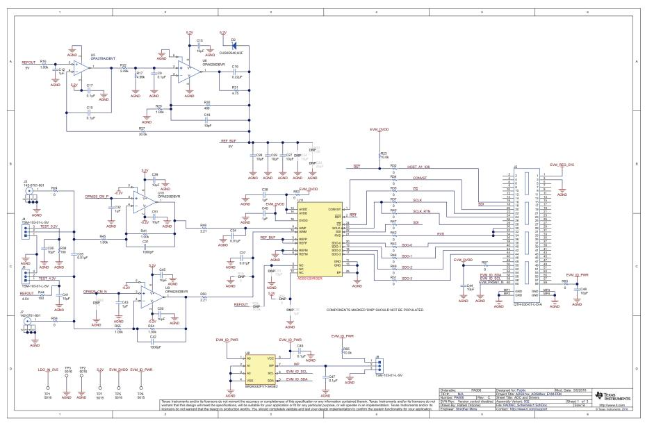
Figure 20. Schematic Diagram (Page 1) of the ADS9120EVM PCB
