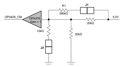
Figure 2. Common-Mode Selection Jumpers
