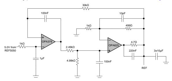
Figure 3. Onboard Reference Signal Path
