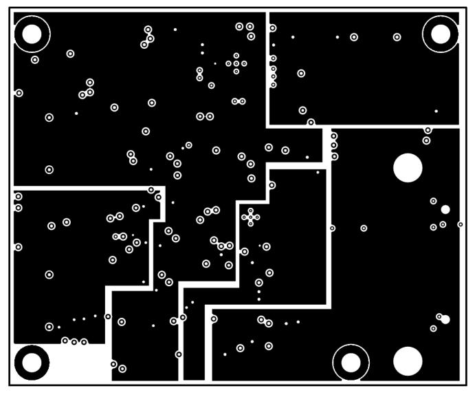
Figure 18. ADS9120EVM PCB Layer 3: Power Planes
