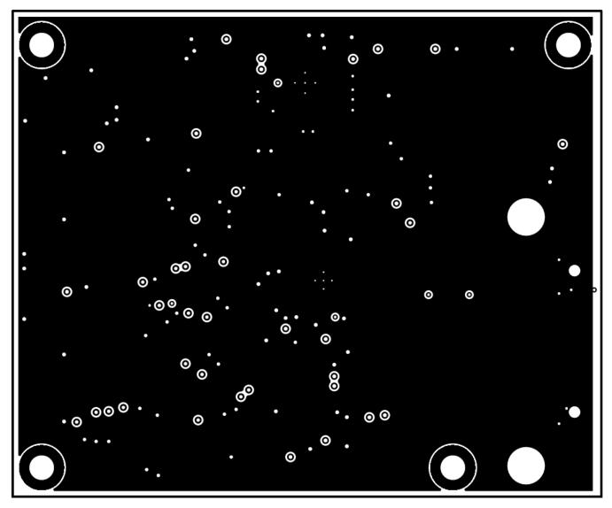
Figure 17. ADS9120EVM PCB Layer 2: GND Plane
