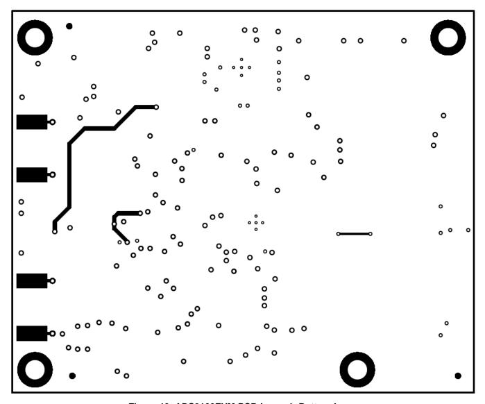
Figure 19. ADS9120EVM PCB Layer 4: Bottom Layer
