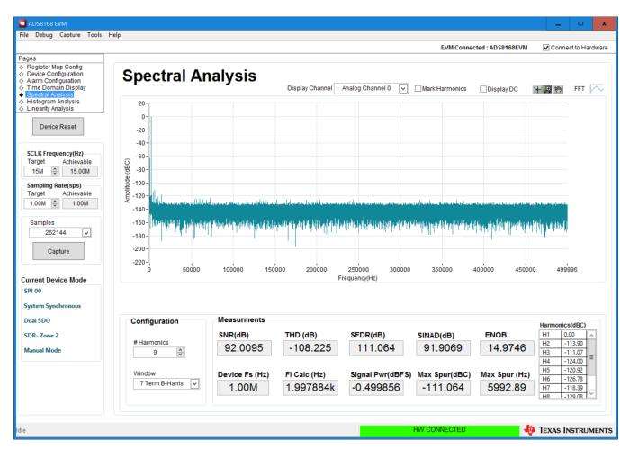
Figure 14. Spectral Analysis Tool
