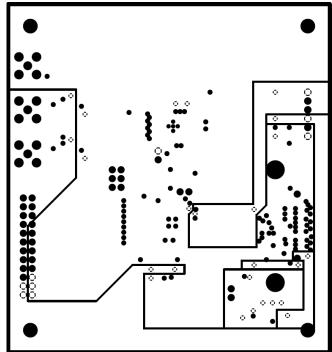
Figure 20. ADS8168 EVM PCB Layer 3: Power Planes
