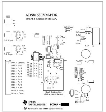
Figure 17. ADS8168 EVM PCB: Top Overlay
