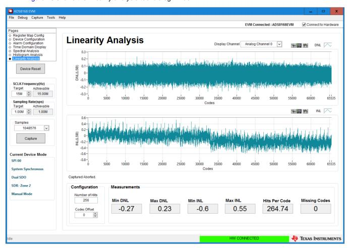
Figure 16. Linearity Analysis Tool
