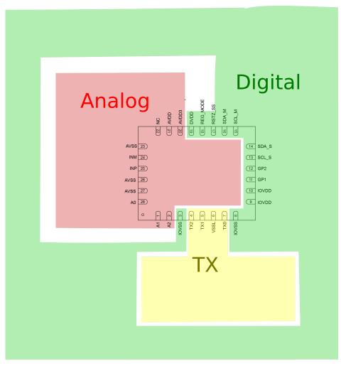
Figure 28. PCB sections recommended
