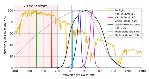
Normalized Spectral Sensitivity(Photodiodes)/Emission(Emitters) for components
