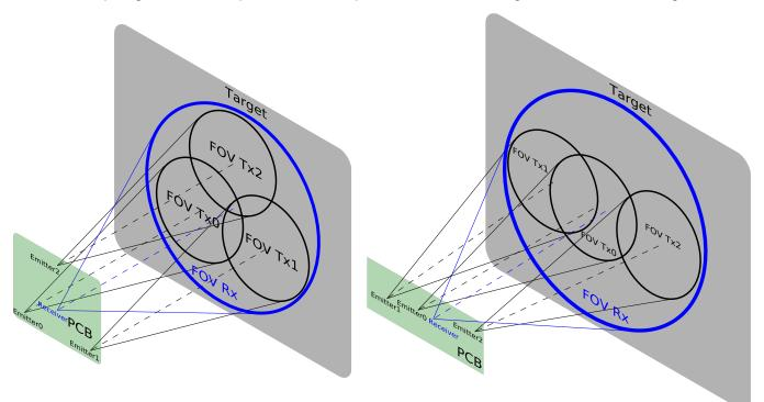
Figure 6. Multi-Zone Arrangement Examples With OPT3101
