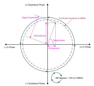
Figure 3. Vector Diagram Representation for ToF Signal
