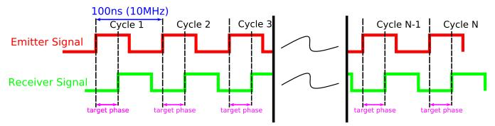
Figure 2. Generic Time-of-Flight Timing Diagram
