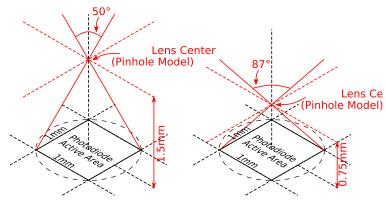
Figure 23. Field of View with pin hole model
