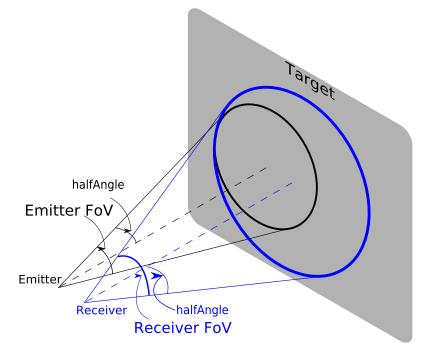
Figure 7. Emitter and Receiver Fields-of-View
