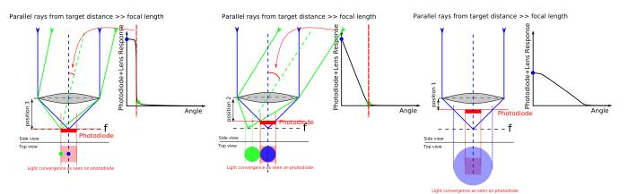
Figure 22. Thin lens ray optics diagram
