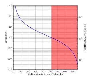
FoV vs Optical gain for 1mm X 1mm photodiode
