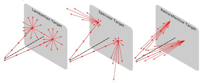
Figure 8. Type of Targets Based on Reflectance
