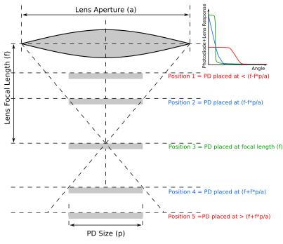
Figure 21. photodiode positioning from lens
