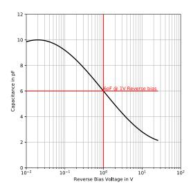
Figure 11. Reverse Biased Junction Capacitance Curve of Photodiode
