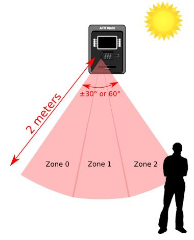
Figure 5. ATM Kiosk person detection system
