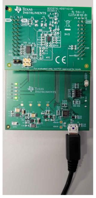
Figure 3-2. BOOSTXL-ADS7142-Q1 Stacked on PAMBoard
