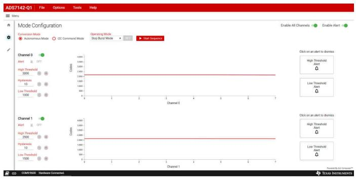
Figure 4-2 highlights the ADS7142-Q1 GUI working in Stop Burst Mode.
