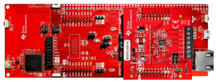
Figure 4. LaunchPad<sup>™</sup> and BoosterPack<sup>™</sup> Combo
