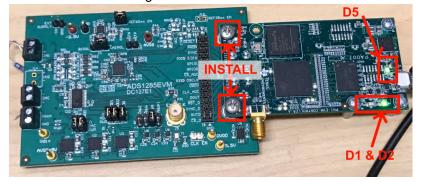
Figure 2-1. ADS1285EVM-PDK Hardware Setup and LED Indicators
