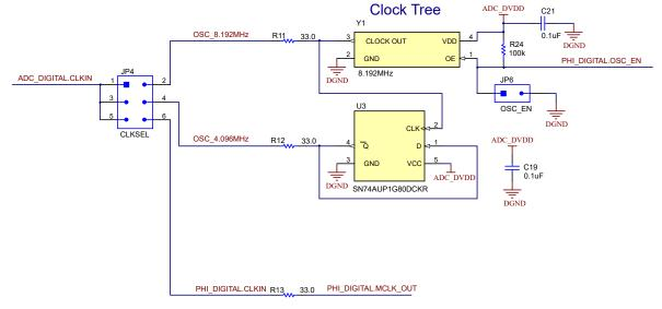
Figure 2-2. Clock Tree (Schematic)
