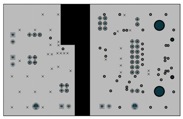
Figure 7-4. Power Layer - Internal
