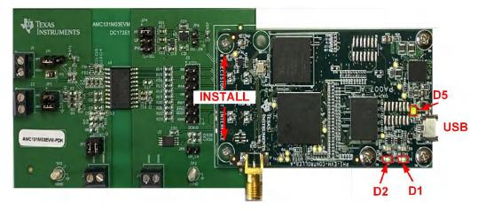
**Figure 6-1. AMC131M03EVM Hardware Setup and LED Indicators** 3. Figure 6-2 shows how to launch the AMC131M03EVM GUI software.
