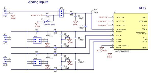
Figure 2-1. Analog Input (Schematic)
