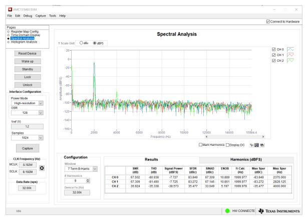
Figure 6-7. Spectral Analysis Tool
