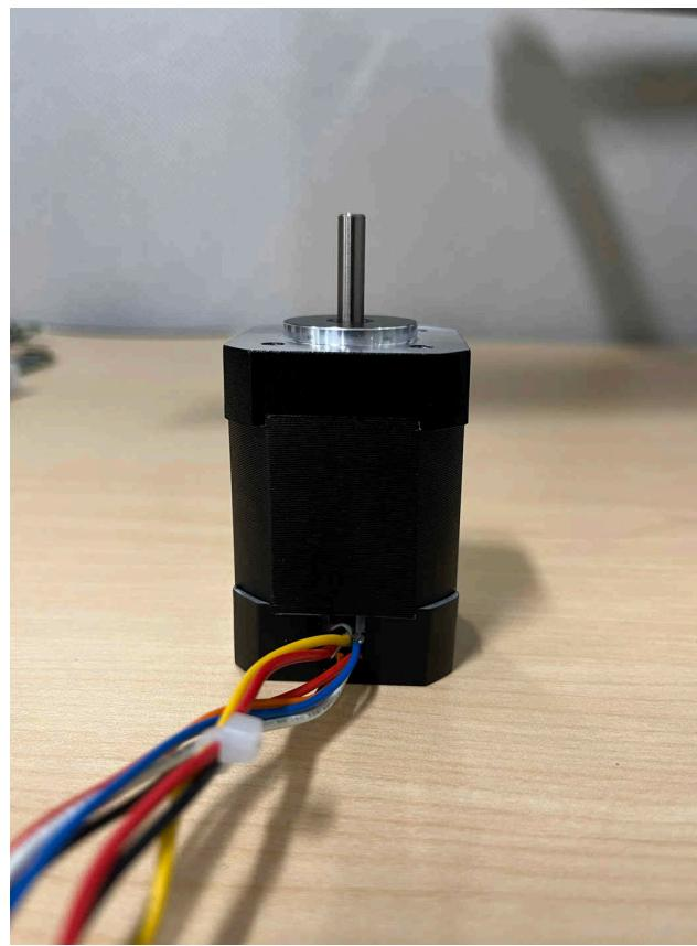
**Figure 3-7. BLDC Motor Connections**
