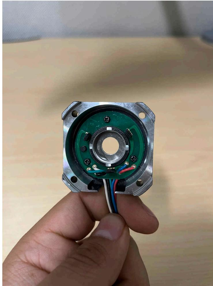
**Figure 3-5. Hall Sensor Board Removal**
