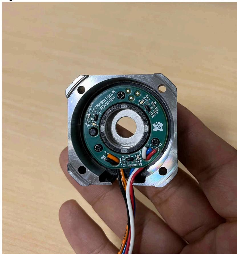
**Figure 3-6. TMAG5115EVM on NEMA17 Motor Module**
