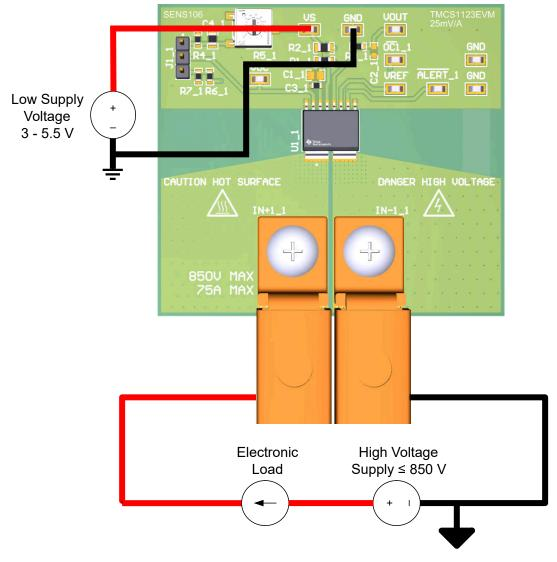
Figure 4-1. Low-Side Forward Current Setup for Reinforced Isolation
