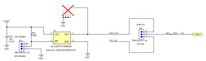
Figure 2-8. Clock Source Circuit
