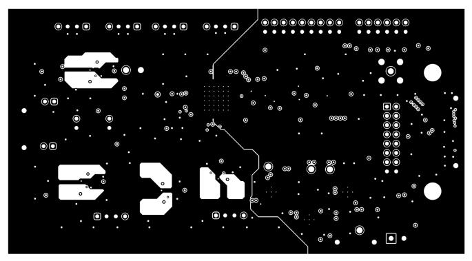
Figure 5-9. Ground Layer Layout
