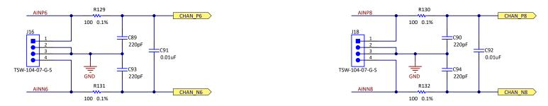
Figure 5-5. Undriven Input Circuitry Schematic
