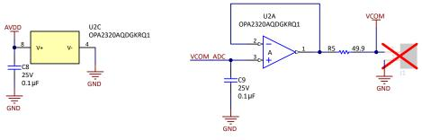
Figure 2-6. VCOM Buffer Circuit
