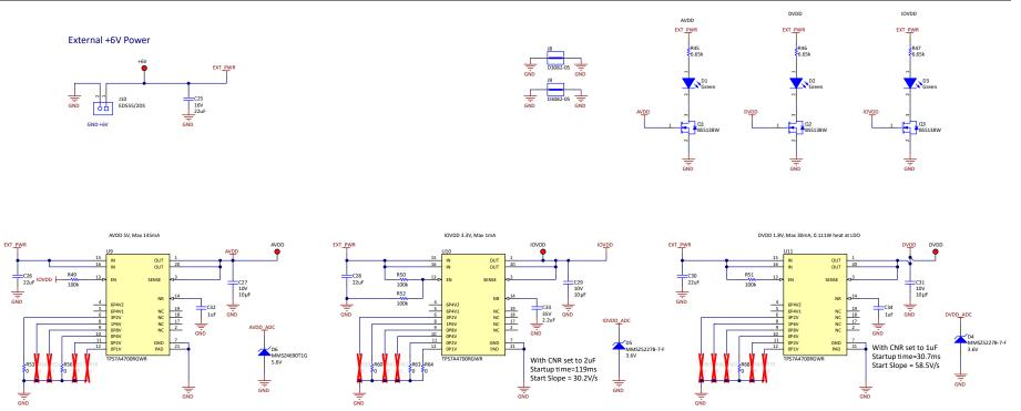
Figure 5-3. Power Supplies Schematic
