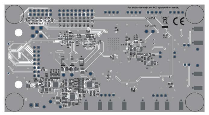
Figure 5-7. Bottom Side Composite Layout
