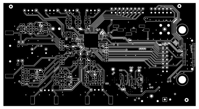
Figure 5-8. Top Signal Layer Layout
