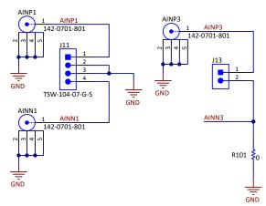
Figure 2-1. SMA Input Connections
