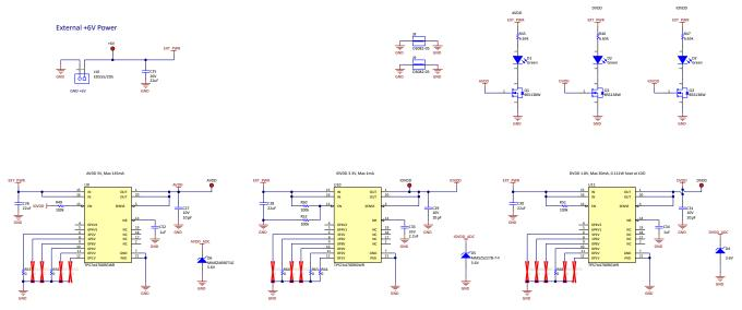
Figure 2-3. Power Supply Circuitry
