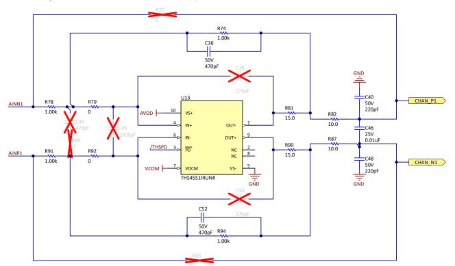
Figure 2-5. Input Drive Amplifier Circuit
