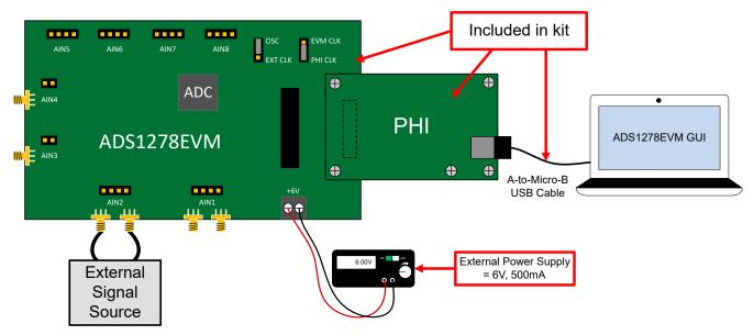
Figure 1-1. System Connection for Evaluation
