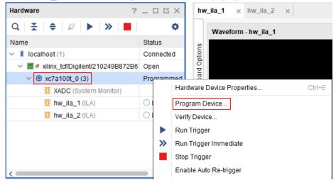
Figure 4-2. Programming FPGA Menu
