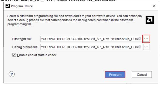
Figure 4-3. Bitfiles to Program FPGA
