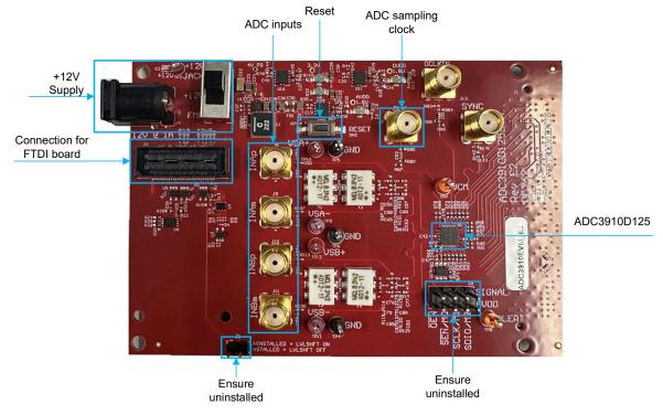
Figure 2-1. ADC3910D125EVM Feature Identification
