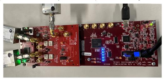
Figure 2-3. Final Setup of ADC3910D125EVM
