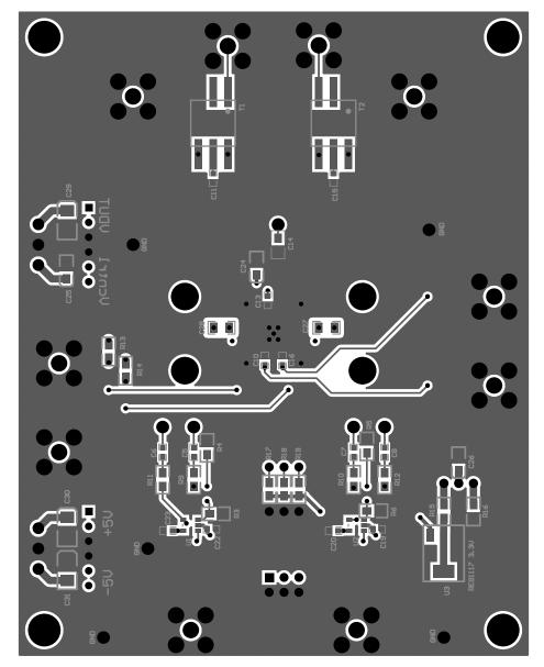
Figure 6. VCA2617EVM PCB Bottom Layer (Bottom View)
