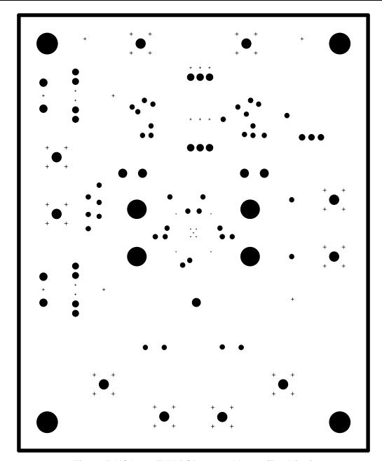
Figure 5. VCA2617EVM PCB Ground Layer (Top View)
