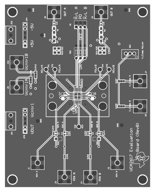
Figure 3. VCA2617EVM PCB Top Layer (Top View)
