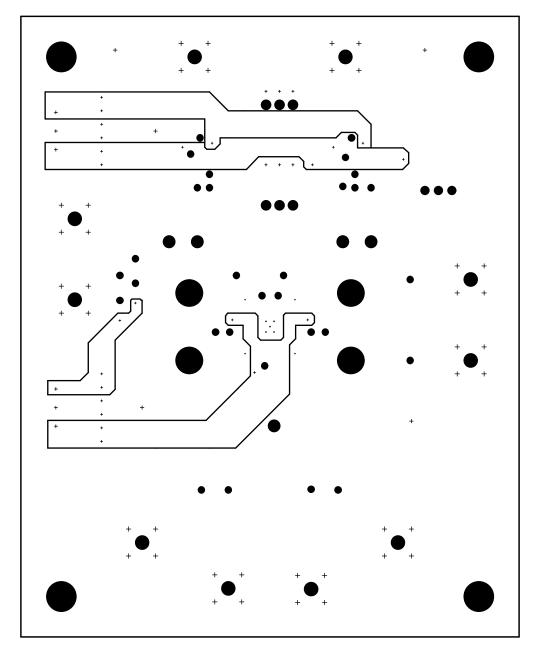
Figure 4. VCA2617EVM PCB Power Layer (Top View)
